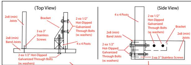
Connection detail of rail post to deck support system for vinyl railing systems that utilize a sleeve which slides over a solid-sawn 4 x 4 post.
