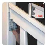
Step 8: Slide the bracket base plate into position, making sure the rail is seated and mark the position of the base plates. Remove the top rail and repeat Step 5.
