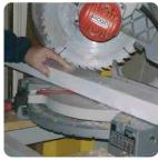
Step 3: For Standard and T-Rail only, subtract 1/8" per side (1/4" total) to allow space for the bracket base plate. Miter cut both the top and bottom rails equally on both sides.
